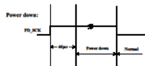
Fig.3 Power down control
